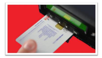
With the chip facing upward and away from you, place the card fully into the tray.
