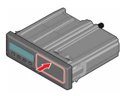
2. Hold the lower edge of the panel and carefully pull out the cassette.
