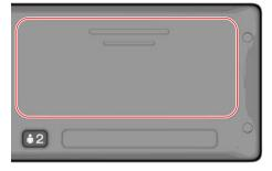
Behind the printer panel there is a printer containing a paper cassette with a paper roll. The printer is used e.g. to make printed records of information stored in the tachograph. The printed paper will come out from a small opening at the bottom of the printer panel.
