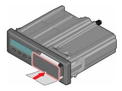
6. Pull the paper upwards and tear it off.
